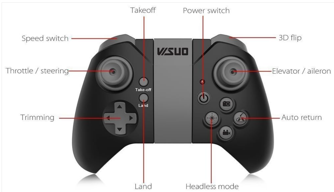
Image: Diagram of the remote controller for the sea jump RC Drone XS809, labeling buttons for Takeoff, Land, Speed switch, Throttle/Steering, Trimming, Power switch, 3D flip, Elevator/Aileron, Auto return, and Headless mode.
