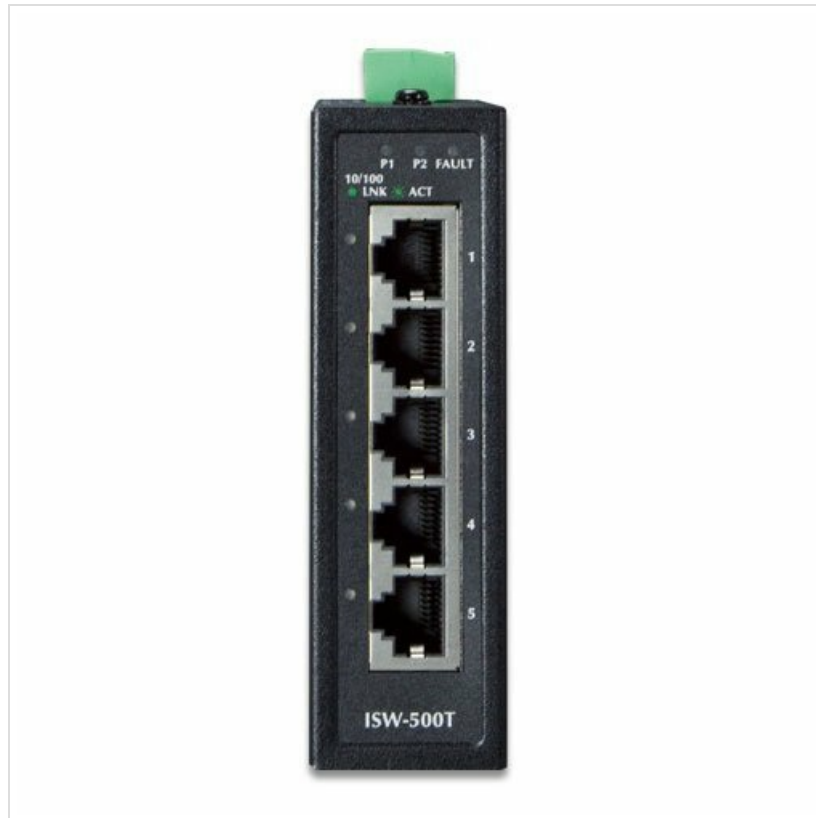
Figure 2.2: Front panel of the ISW-500T, detailing the five 10/100TX Ethernet ports (labeled 1-5) and LED indicators for power (P1, P2), fault (FAULT), and link/activity (LNK/ACT).
