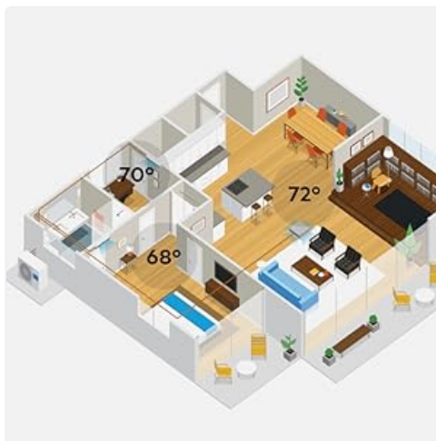
Image: A floor plan illustration demonstrating how the dual-zone system can maintain different temperatures in various rooms, such as 70°F, 72°F, and 68°F, highlighting independent zone control.
