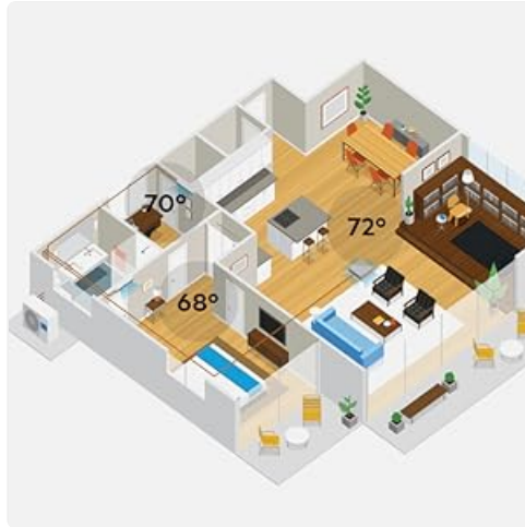
Image: An isometric floor plan demonstrating how different rooms can maintain distinct temperature settings using a multi-zone mini-split system.
