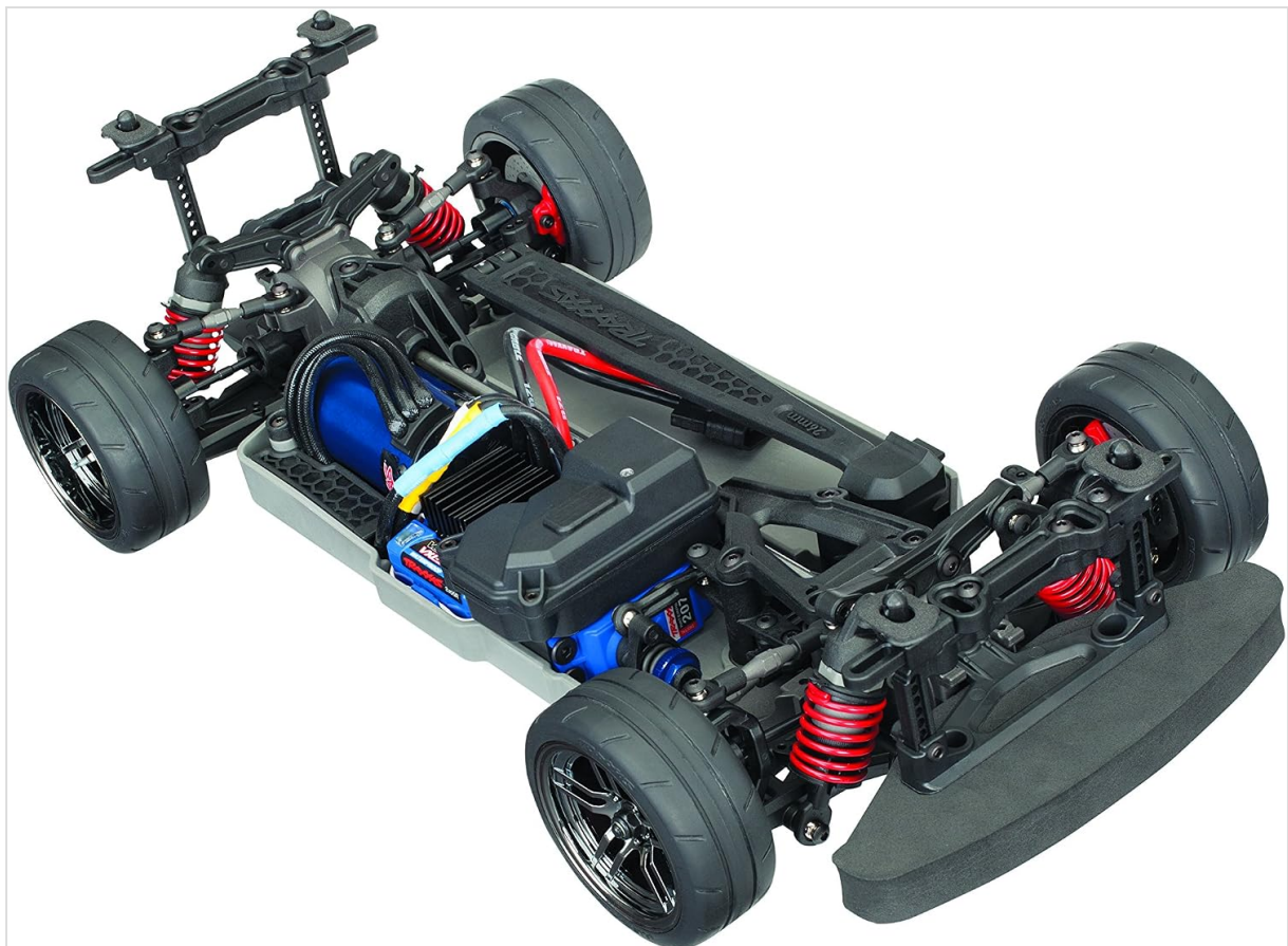
Figure 2: Overview of the Traxxas 4-Tec 2.0 VXL chassis, showcasing its modular design and components.
