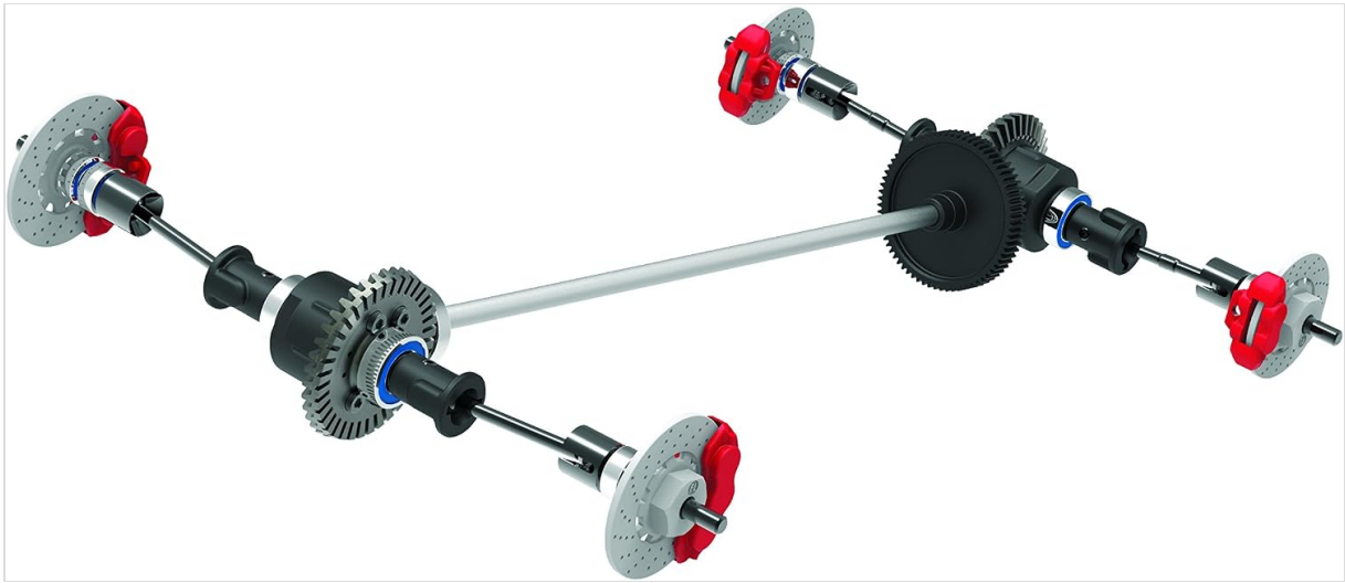
Figure 7: Diagram illustrating the all-wheel-drive (AWD) drivetrain system.
