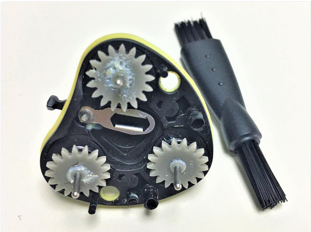
Figure 2: Underside view of the Shaver Head Motor Drive Shaft Axis assembly, illustrating the gear mechanism that connects to the shaver's motor, alongside the cleaning brush.
