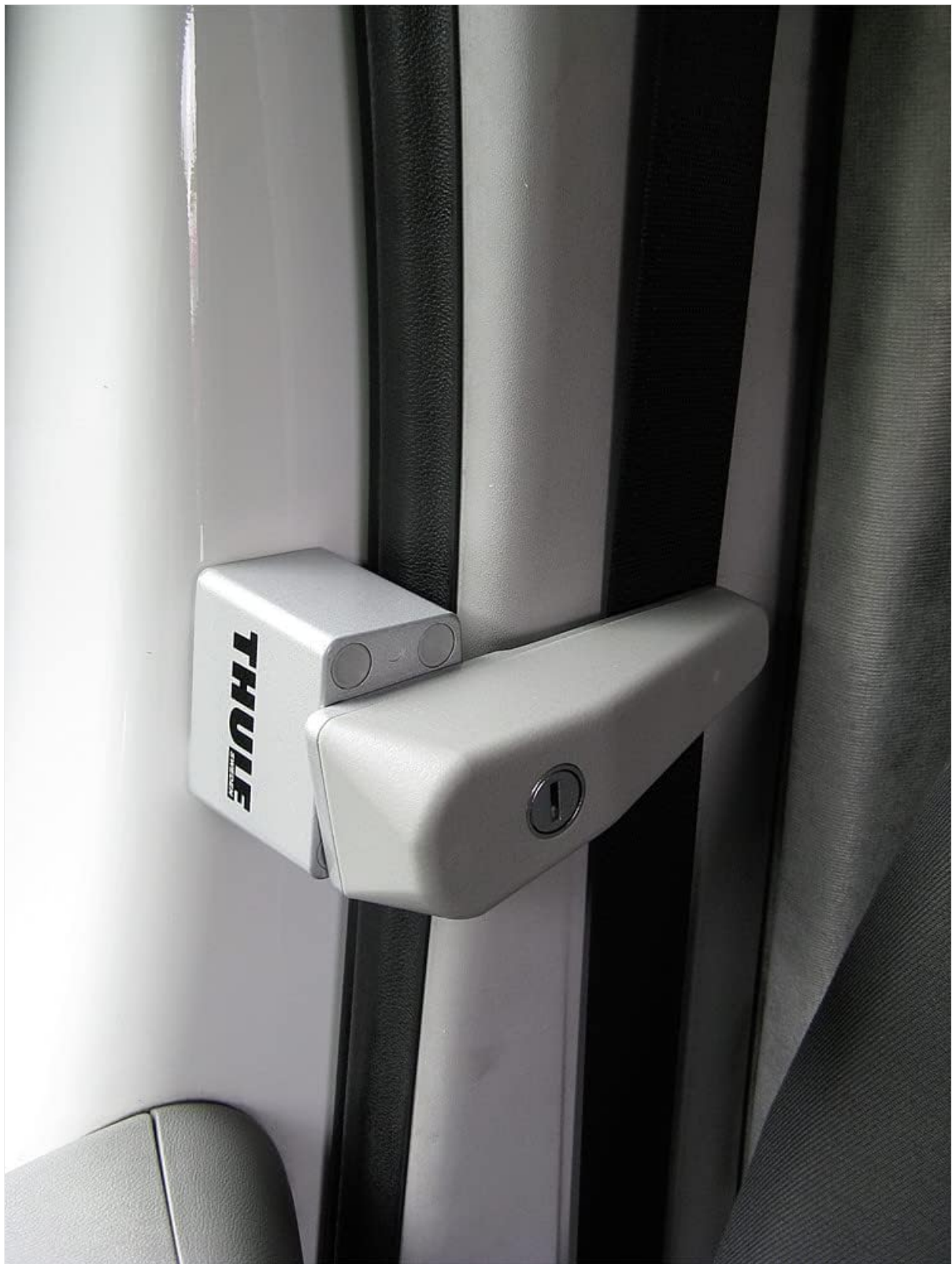
Image: The Thule RV Cab Lock shown installed on the interior of a vehicle cabin door, demonstrating its position and function.
