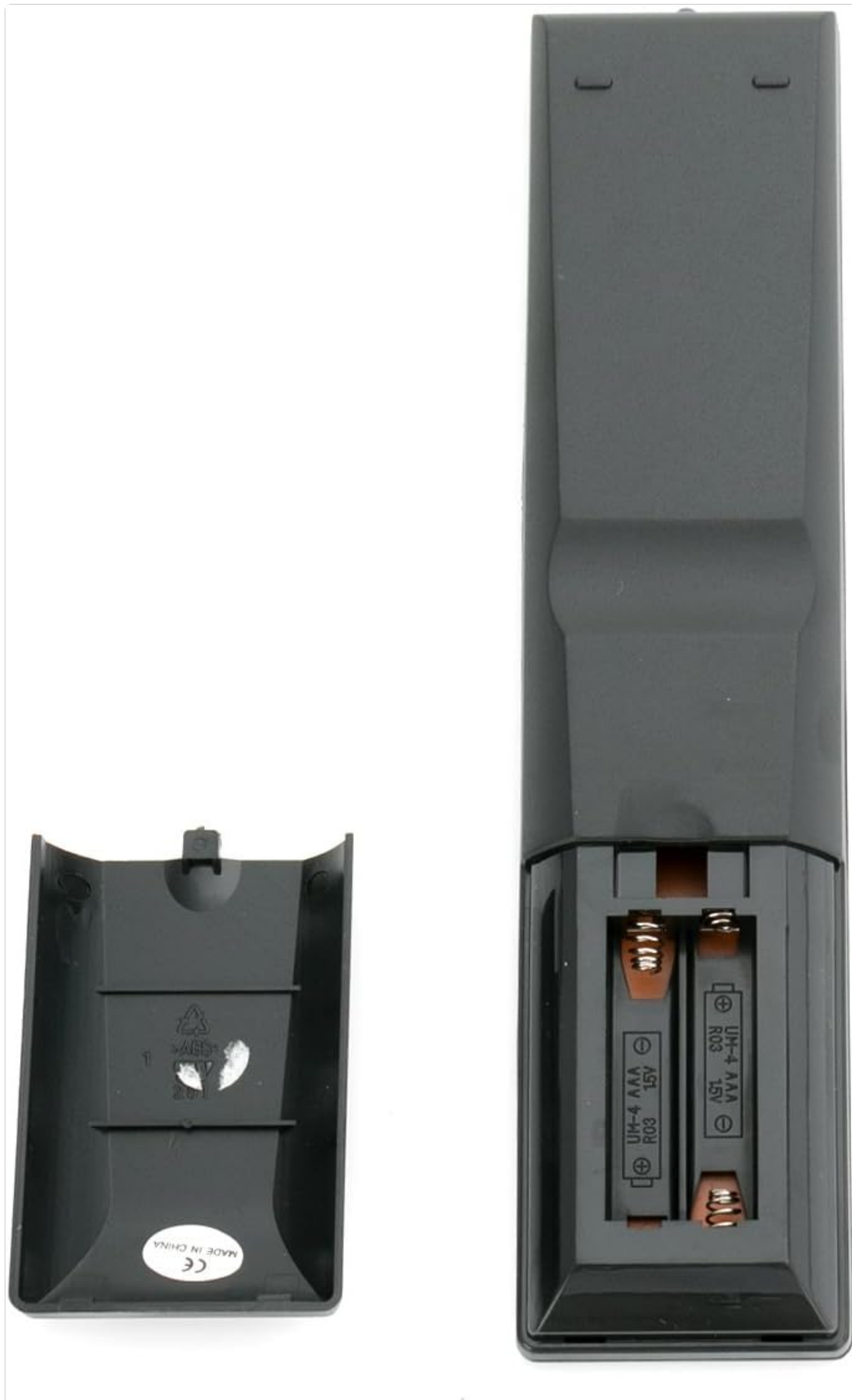
Figure 2: Back view of the remote control with the battery compartment open, illustrating the correct orientation for AAA battery insertion.
