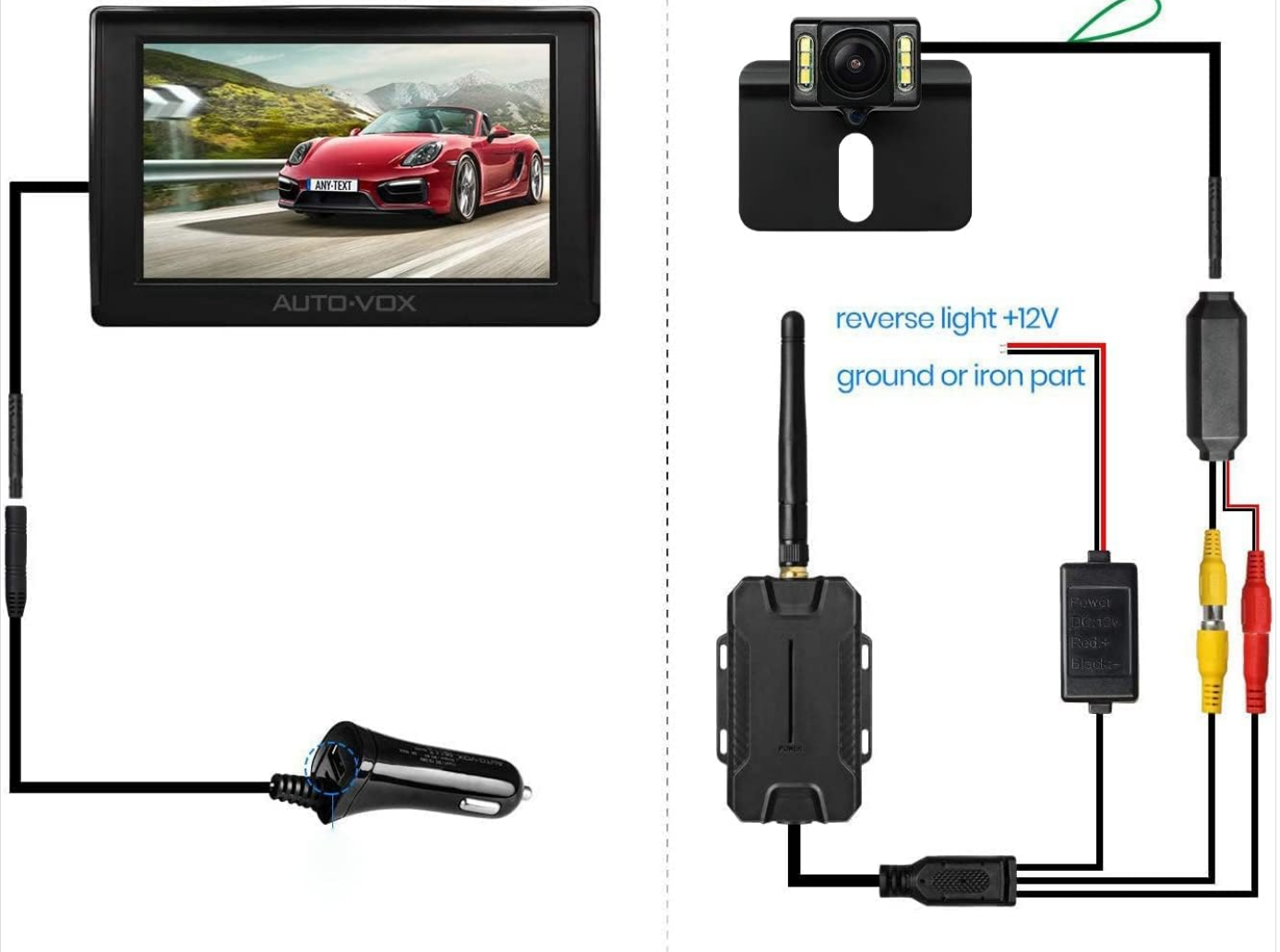
Figure 3: Simplified wiring diagram for the camera and monitor setup.
