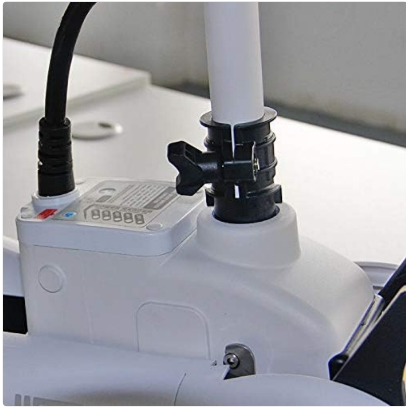
Figure 2.3.2: The depth adjustment collar allows users to set the desired motor depth in the water.
