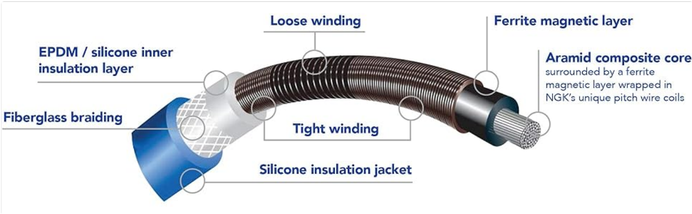
Image 2.1: Cross-section diagram of an NGK spark plug wire.
