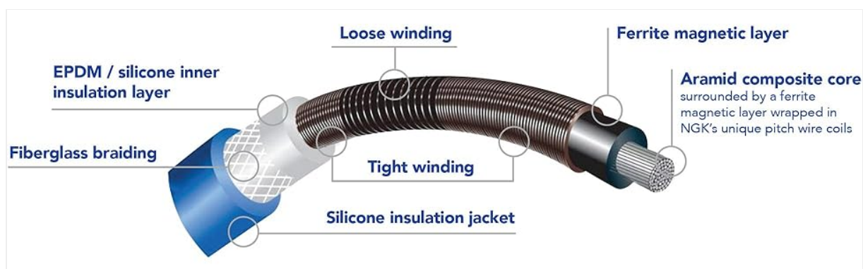
Image 2: Detailed diagram showing the internal components of an NGK spark plug wire, including the EPDM/silicone inner insulation, fiberglass braiding, loose and tight winding, ferrite magnetic layer, and aramid composite core.
