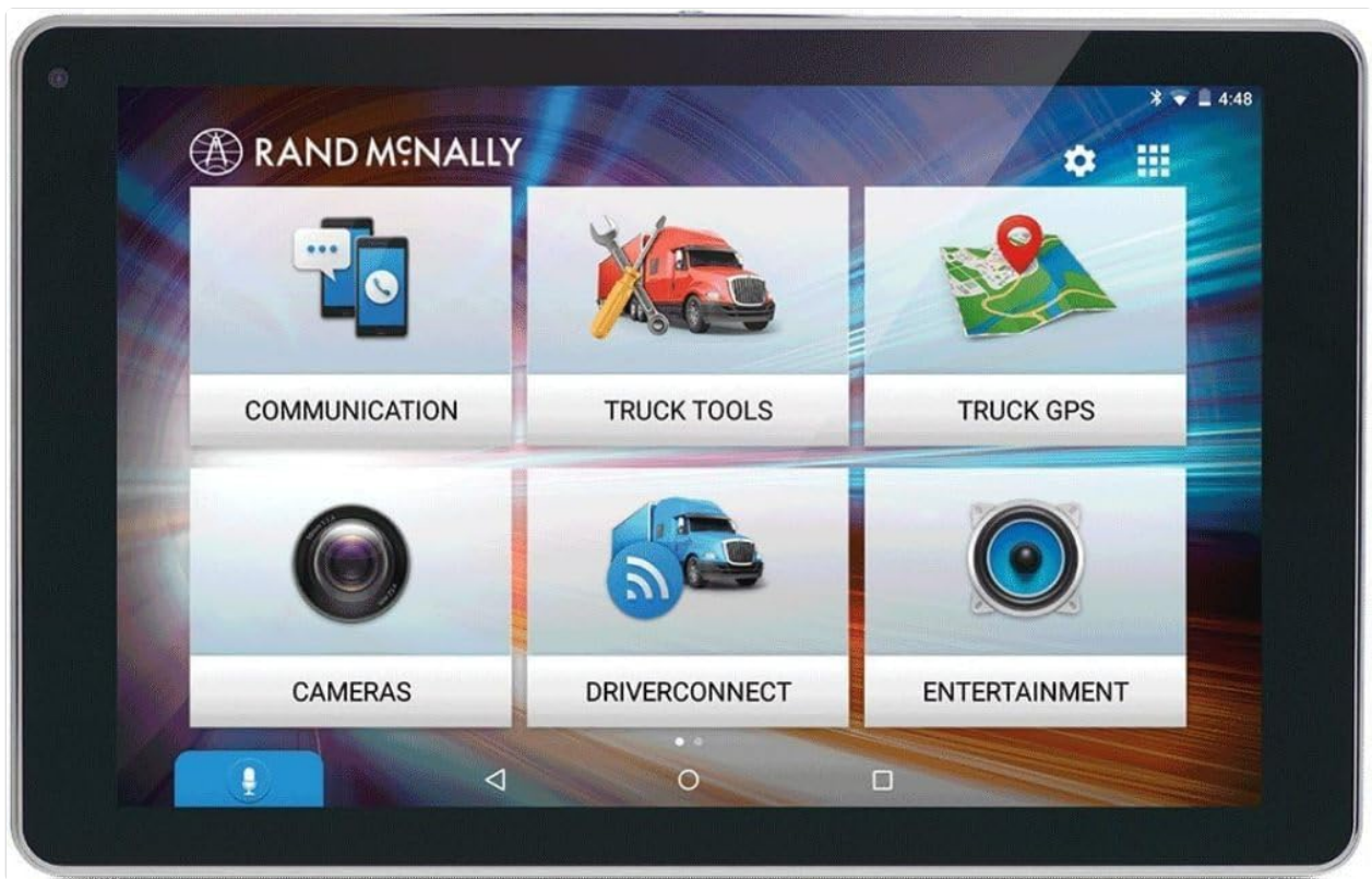
Image: The home screen of the OverDryve 8 Pro tablet, displaying six primary application icons for navigation, communication, and other truck-specific tools.
