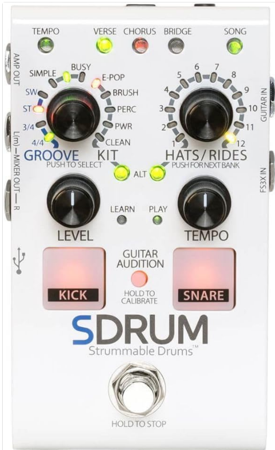
Figure 1: Top view of the DigiTech SDRUM pedal, highlighting its various controls and the main footswitch.
