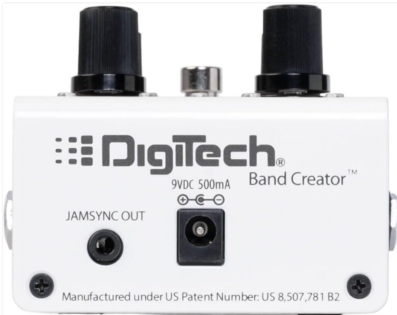
Figure 2: Rear view of the SDRUM, illustrating the power input and JamSync Out port.
