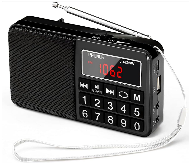
Figure 2.1: Front view of the PRUNUS J-429 Portable Radio, showing the speaker grille, digital display, numeric keypad, and control buttons.
