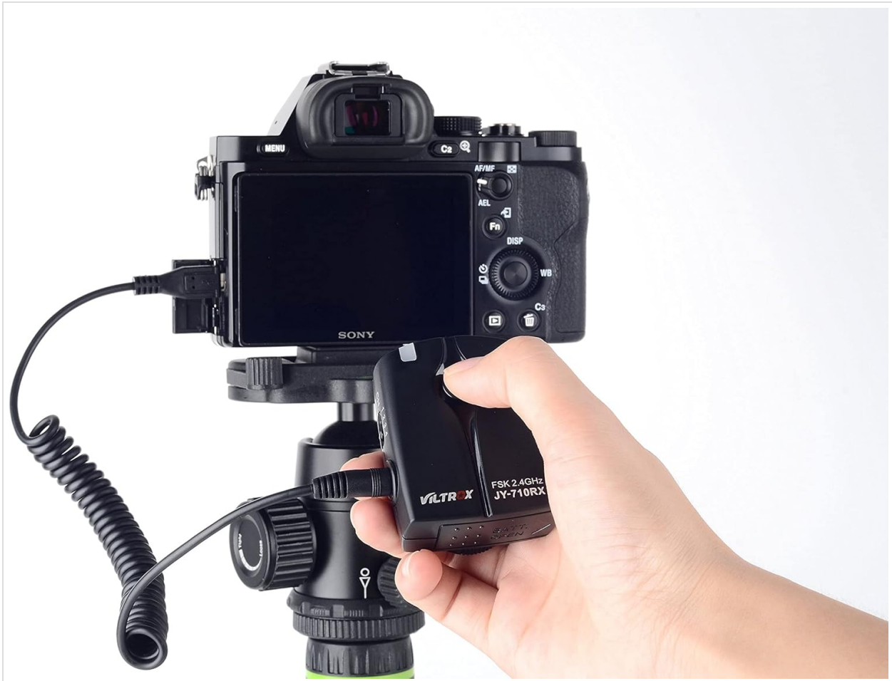
Image 2: Transmitter connected directly to a Sony camera for wired operation.
