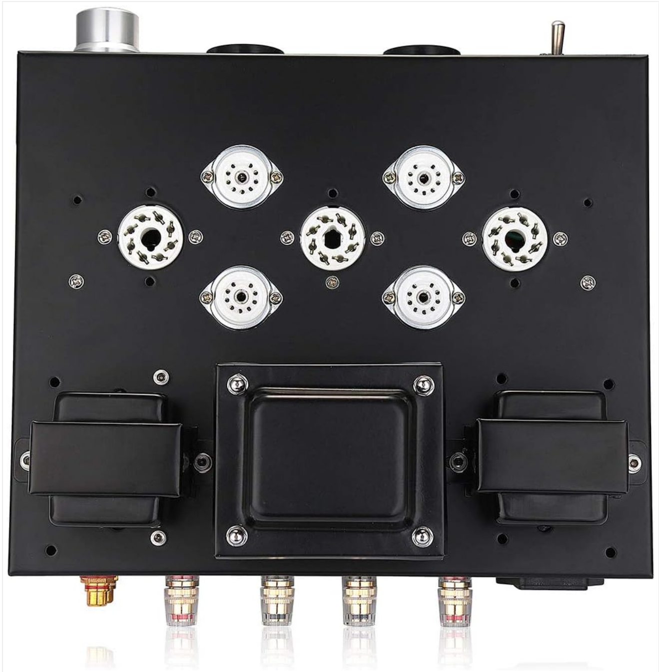
Figure 4.1: Underside view of the amplifier, illustrating the arrangement of tube sockets for proper tube installation.
