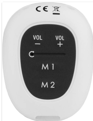
Figure 4.5: Rear view of the SOS medallion, showing the volume controls and M1/M2 direct dial buttons.
