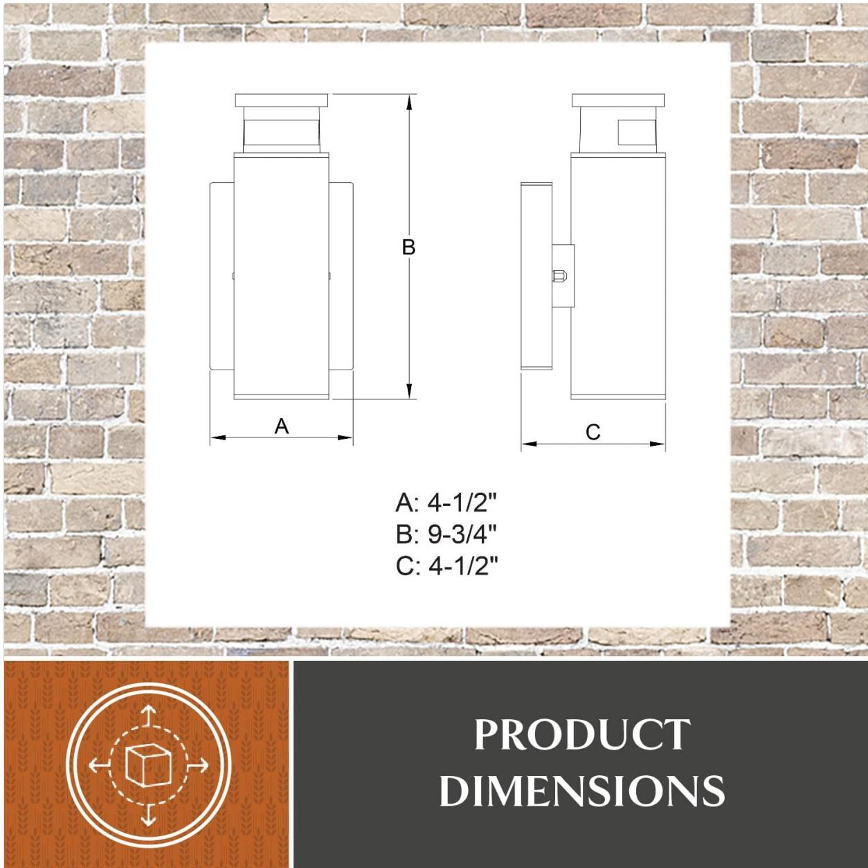
This diagram illustrates the key dimensions of the VAXCEL Chiasso T0344 wall sconce, with measurements A, B, and C indicating width, height, and depth respectively.
