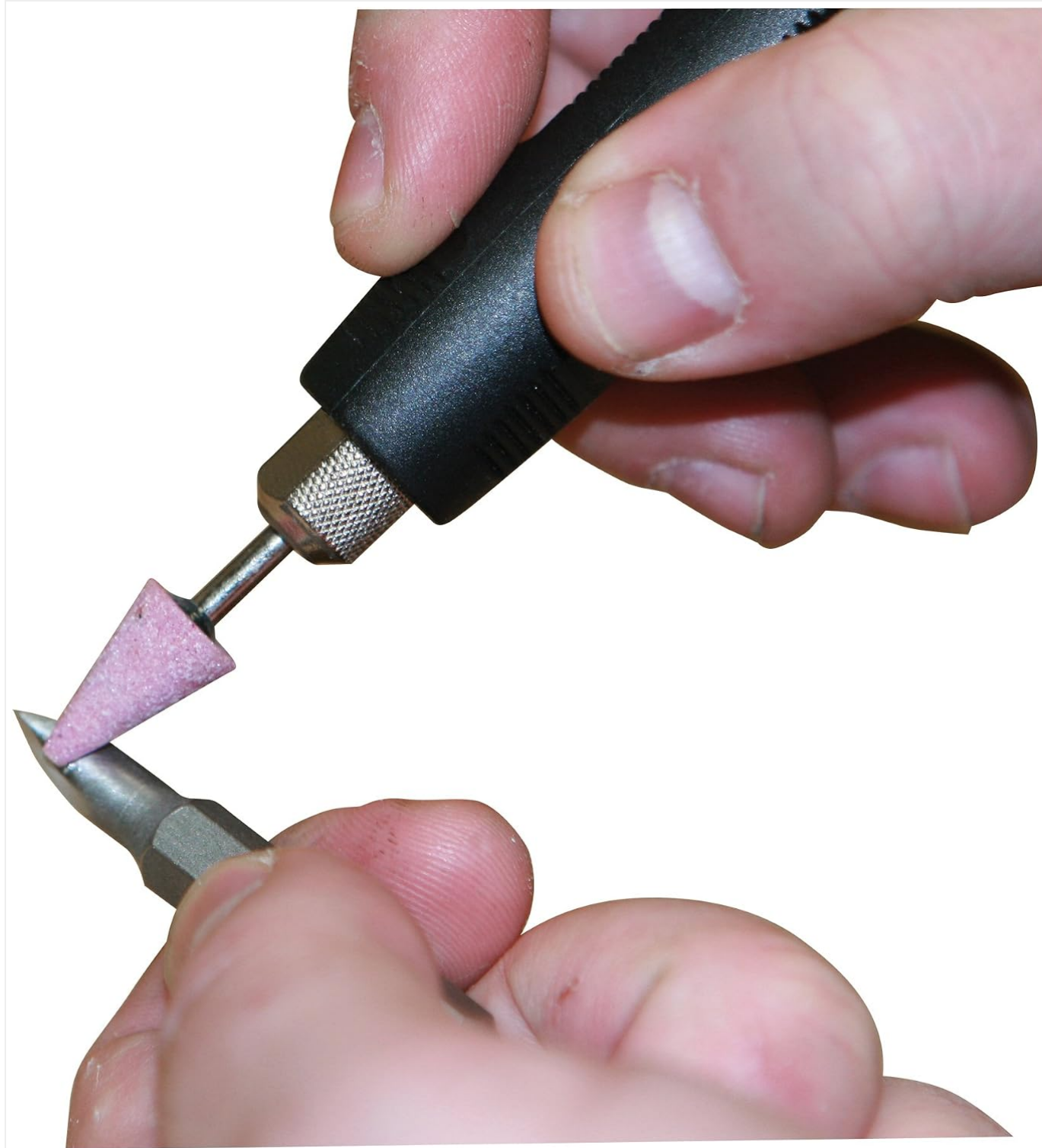
Figure 5: A user demonstrating the flexible shaft with a grinding stone for fine carving on a metal part, highlighting its precision capabilities.
