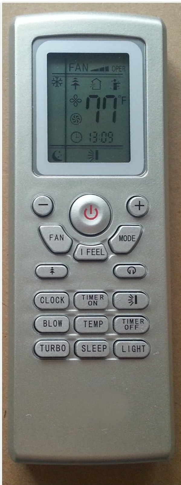
Figure 4.2: Close-up of the remote control's LCD display, showing temperature, fan speed, and mode indicators.
