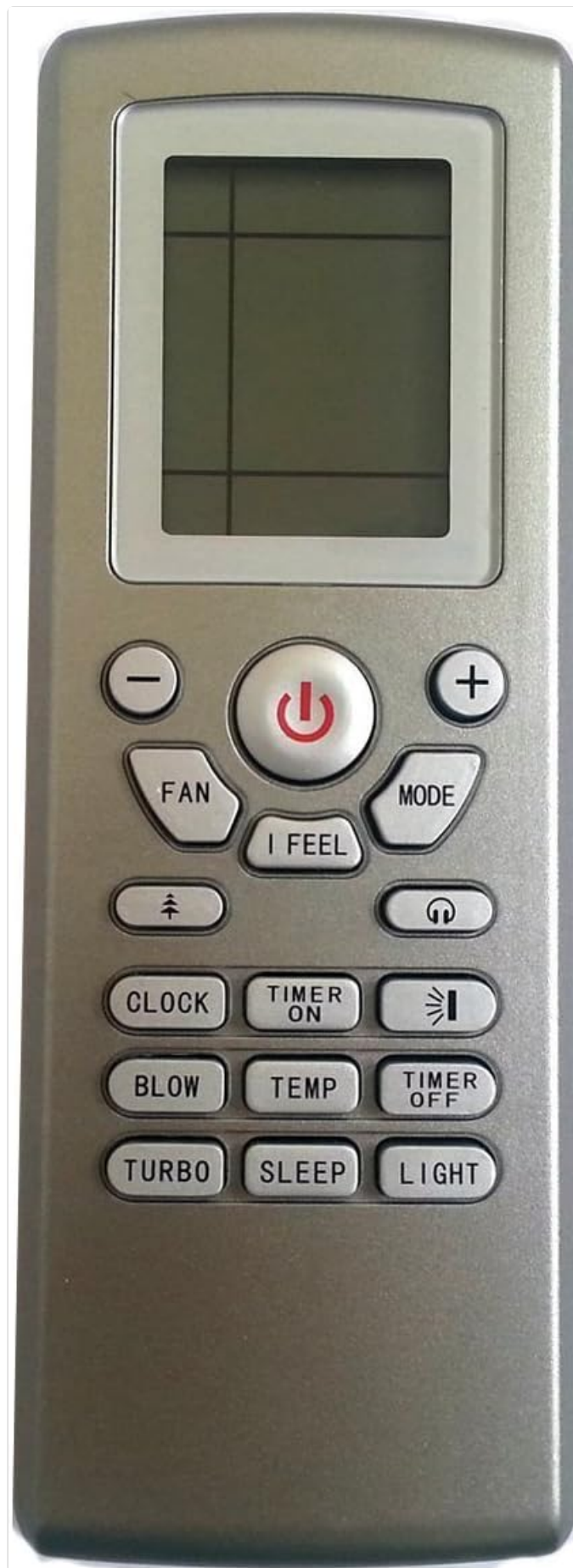
Figure 4.1: Detailed view of the GREE YB1F Remote Control, showing all buttons and the display screen.
