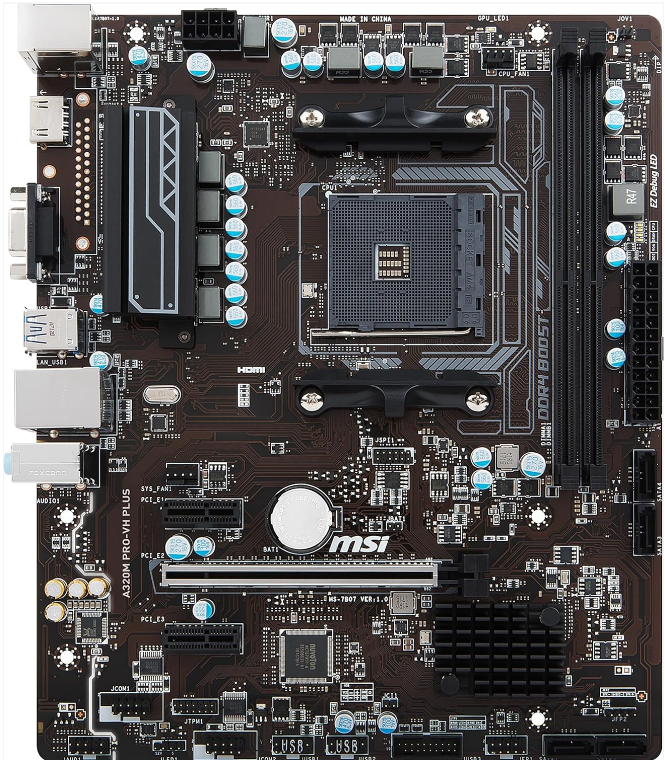
Image: A top-down view of the MSI A320M PRO-VH PLUS motherboard, showing the CPU socket (AM4) at the center, surrounded by mounting holes for the CPU cooler.
