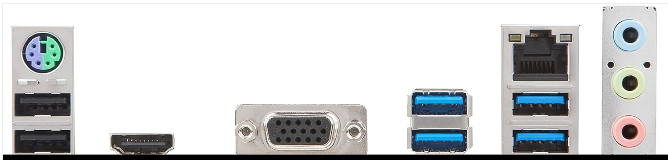
Image: A close-up view of the rear input/output (I/O) panel of the MSI A320M PRO-VH PLUS motherboard, showing various ports including PS/2, USB, HDMI, VGA, LAN, and audio jacks.
