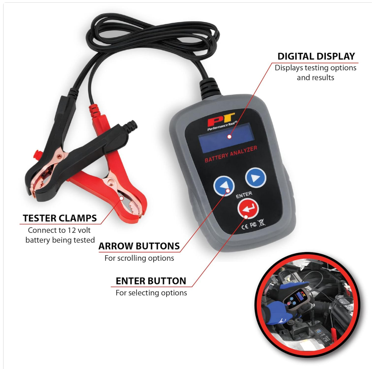
Figure 2: Key components of the W2998 Battery Analyzer.
