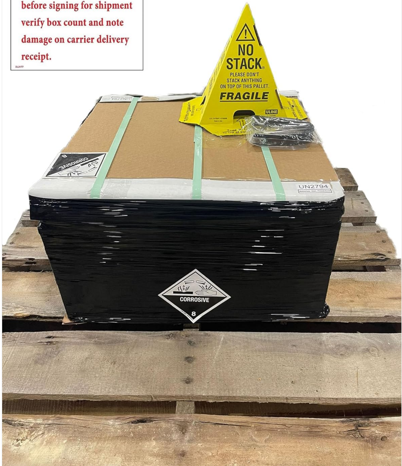
Figure 2.1: Palletized shipment of batteries with a 'NO STACK' warning and corrosive material labels. Always inspect for damage before accepting delivery.
