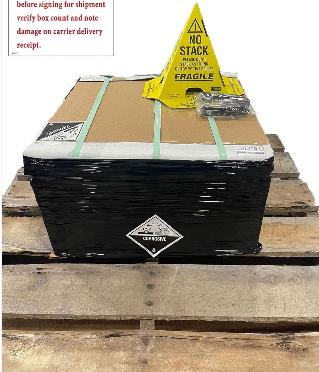
Image 4.1: Palletized shipment of batteries, displaying 'NO STACK' and 'CORROSIVE' hazard warnings, emphasizing the importance of careful handling and inspection upon delivery.
