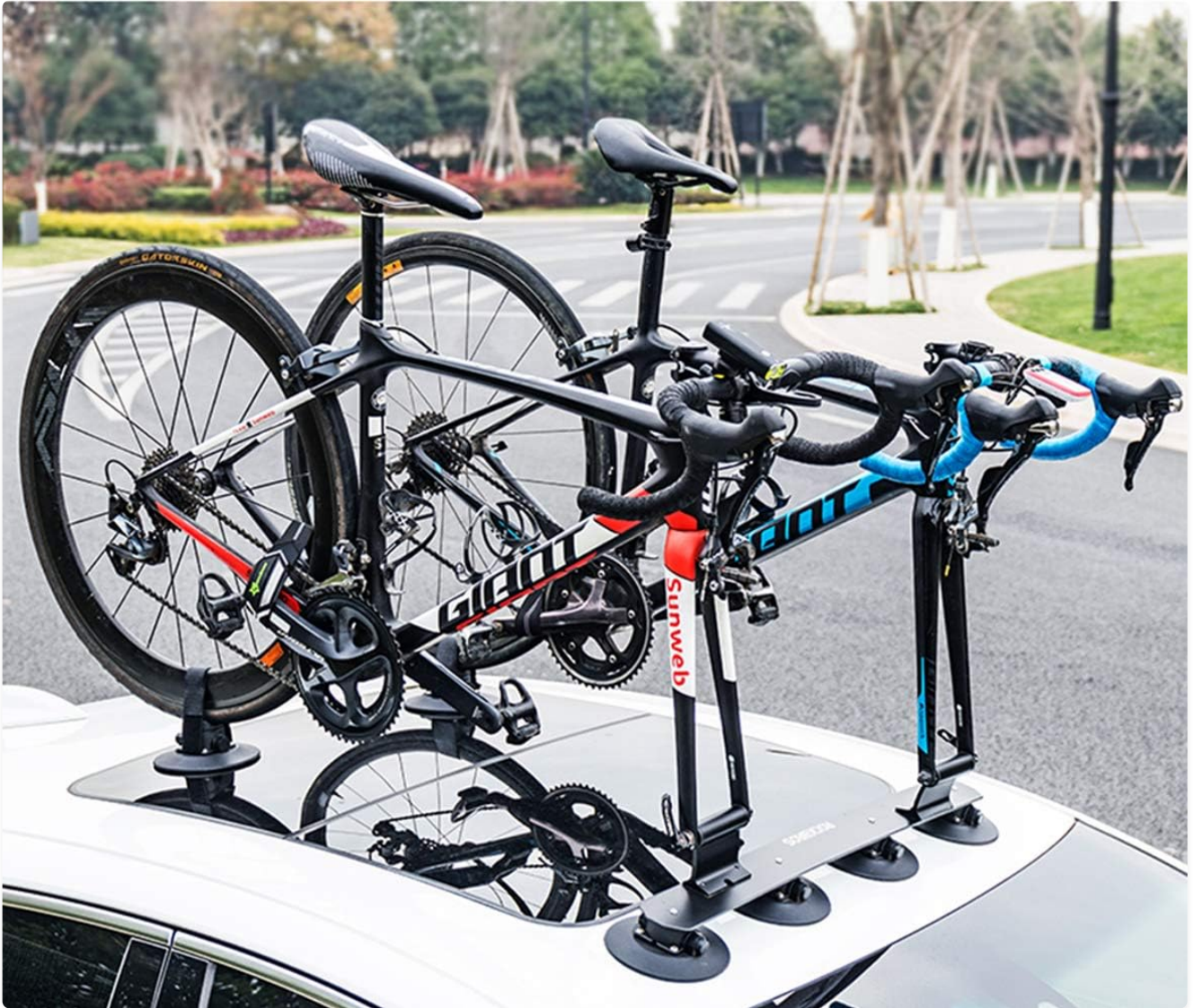
Figure 5: Example of a bike securely mounted on a car roof using the suction cup rack.
