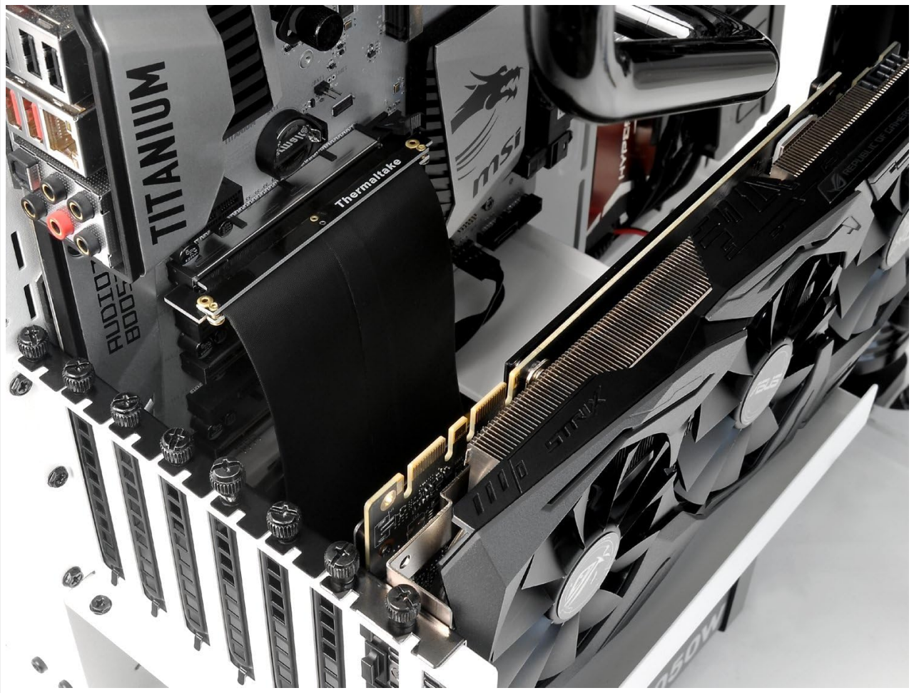
Figure 3.6: Another view of the riser cable installed, demonstrating cable routing within the chassis.
