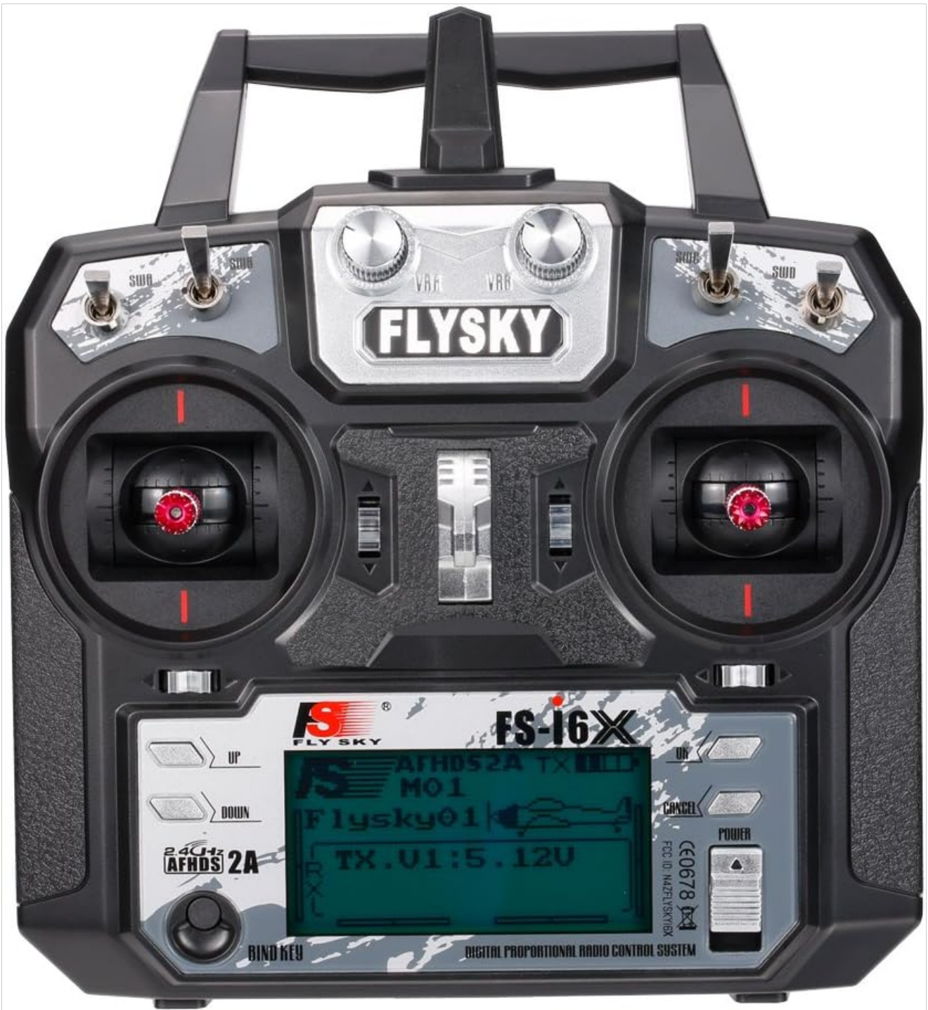
Figure 1.1: Front view of the FS-i6X Transmitter, showing the dual joysticks, LCD screen, and various switches.
