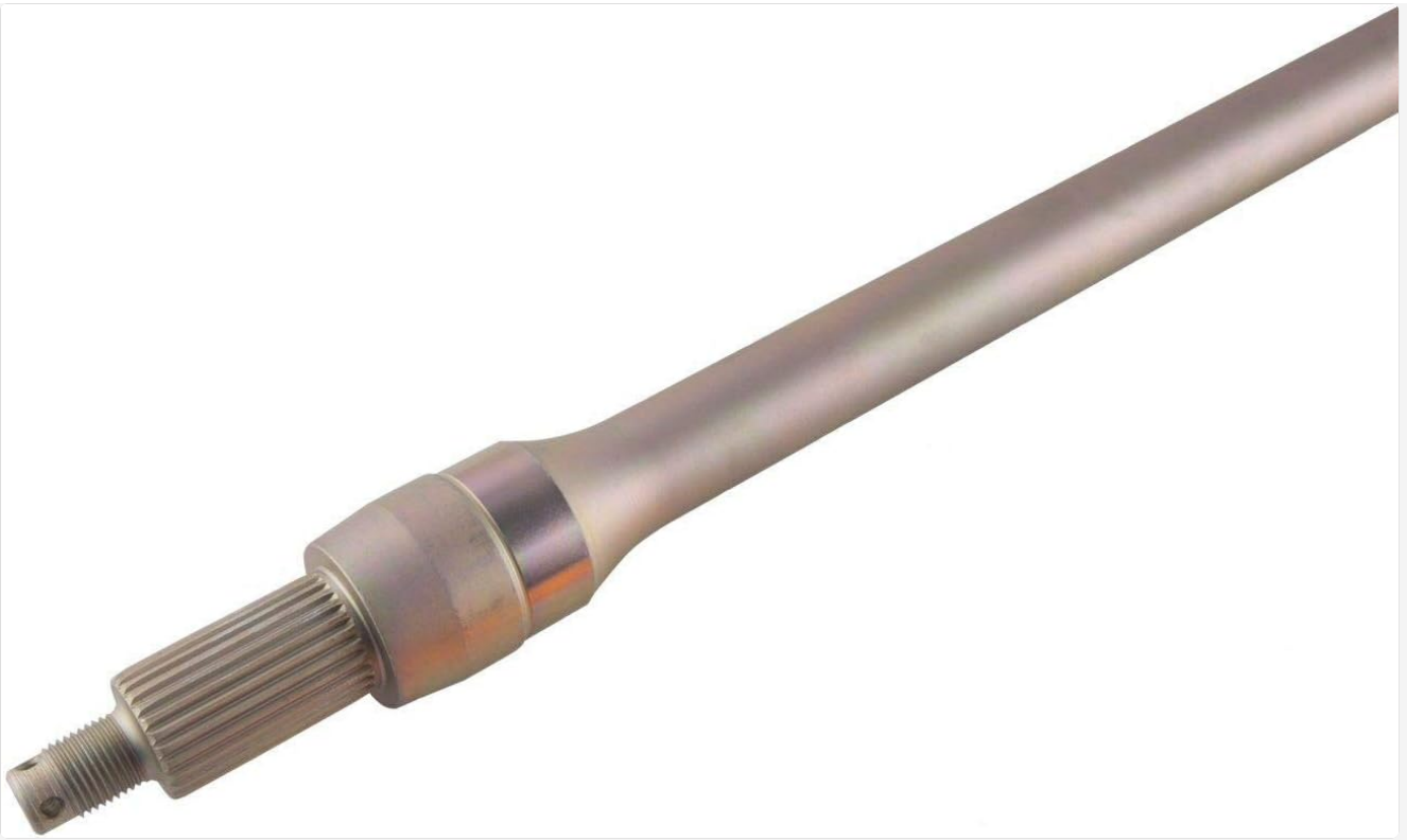
Image 5.1: Close-up view of one spline end of the axle, which connects to the wheel hub.
