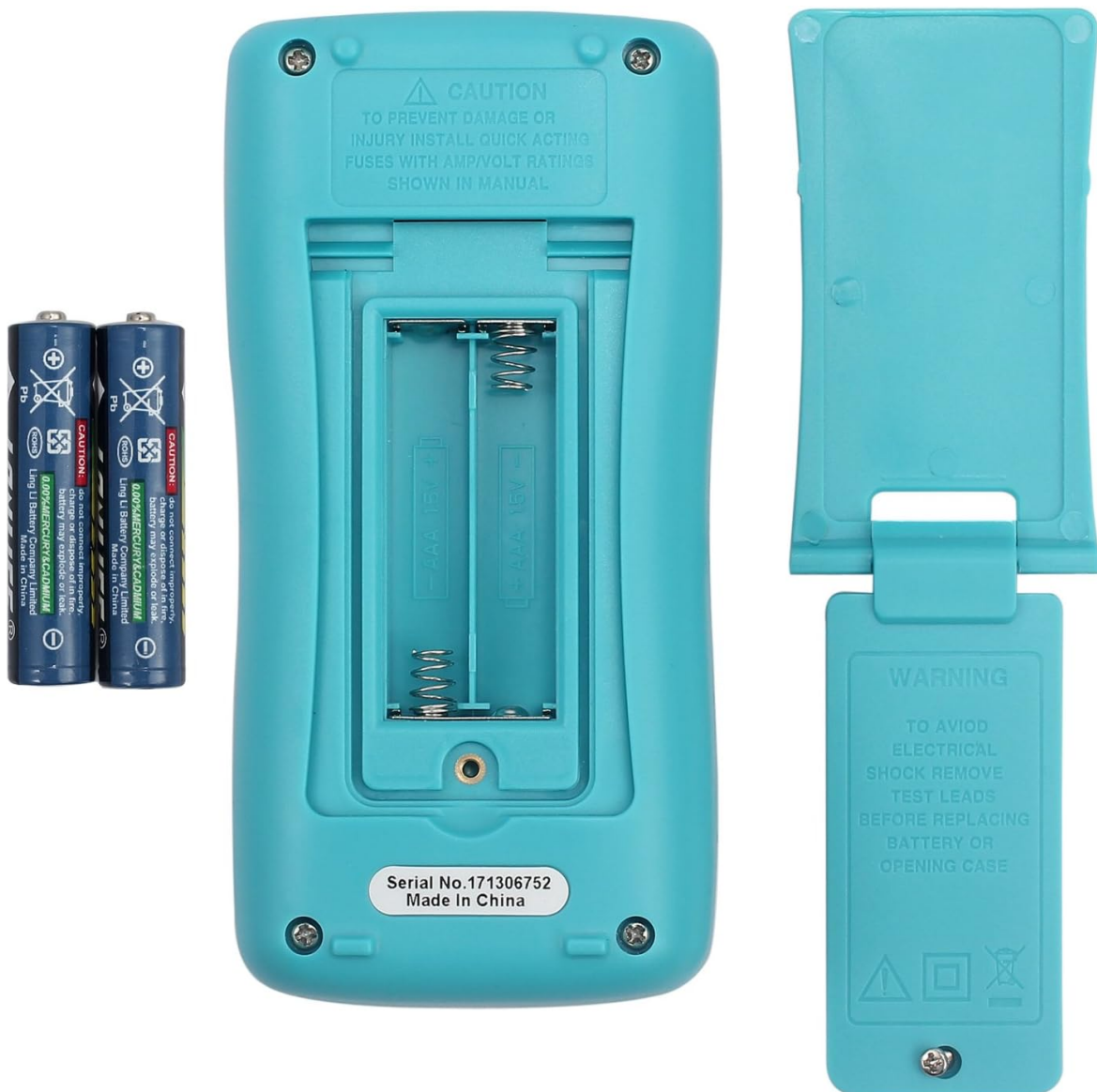
Figure 6.1: Battery compartment on the back of the multimeter.
