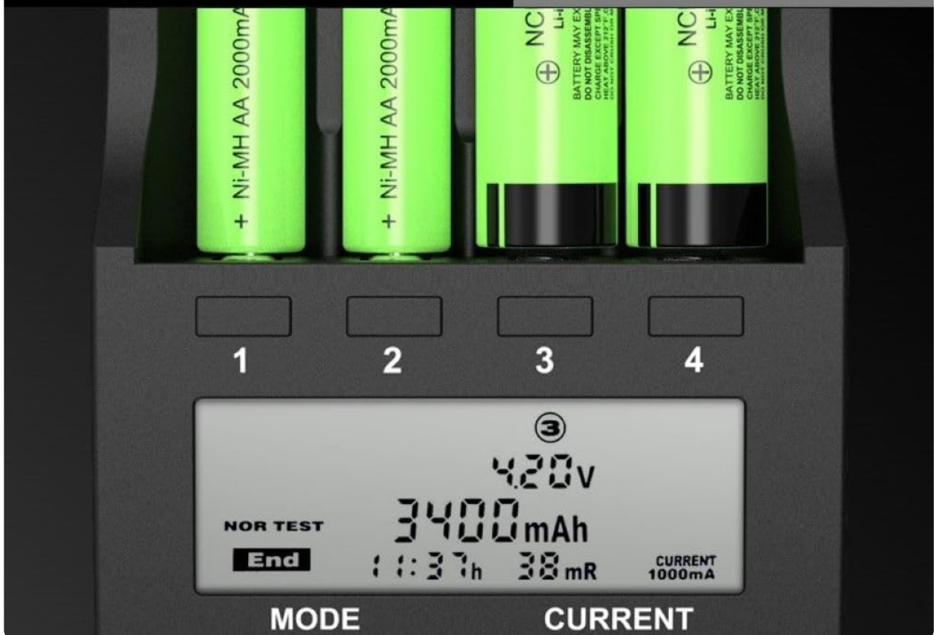
Image: The charger's LCD display showing 'NOR TEST' in progress, indicating the measured capacity and elapsed time.
