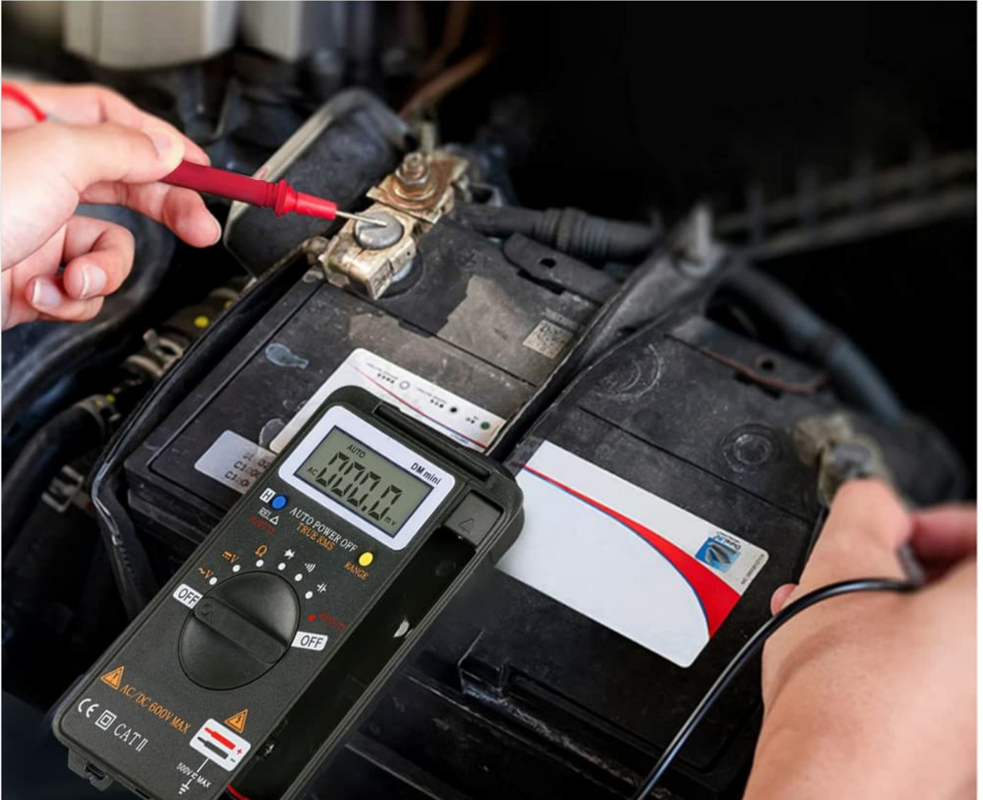
Figure 4.2: The multimeter in use, demonstrating its ease of operation for various electrical tests, such as checking a car battery.
