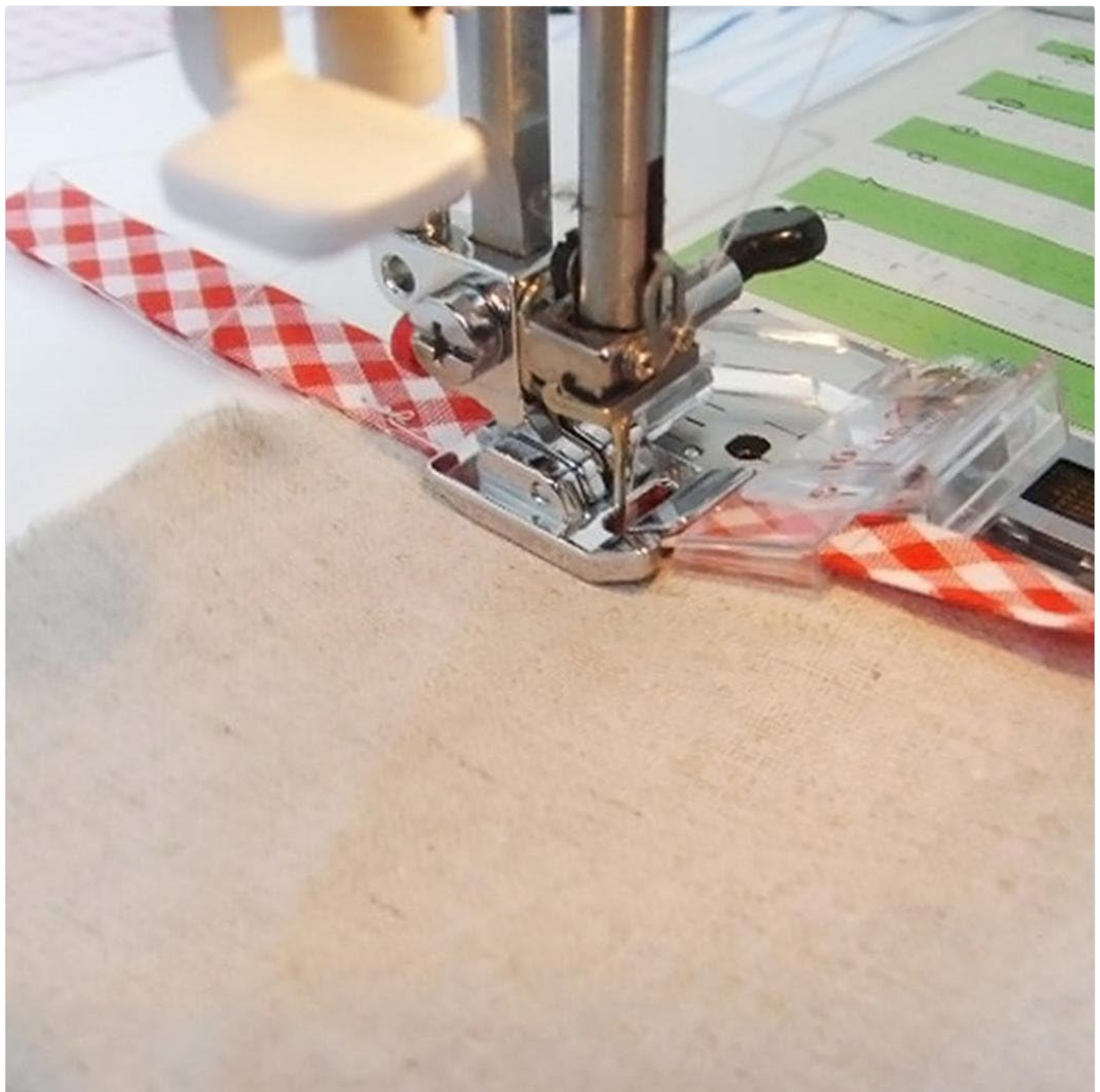
Image 1.1: The YEQIN Adjustable Tap Bias Binder Foot, showing its construction.
