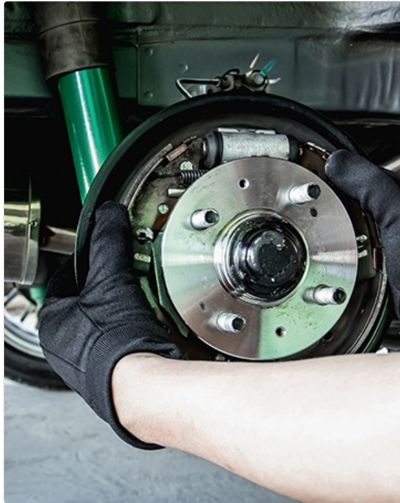
Figure 8: Cleaning the Hub Surface
