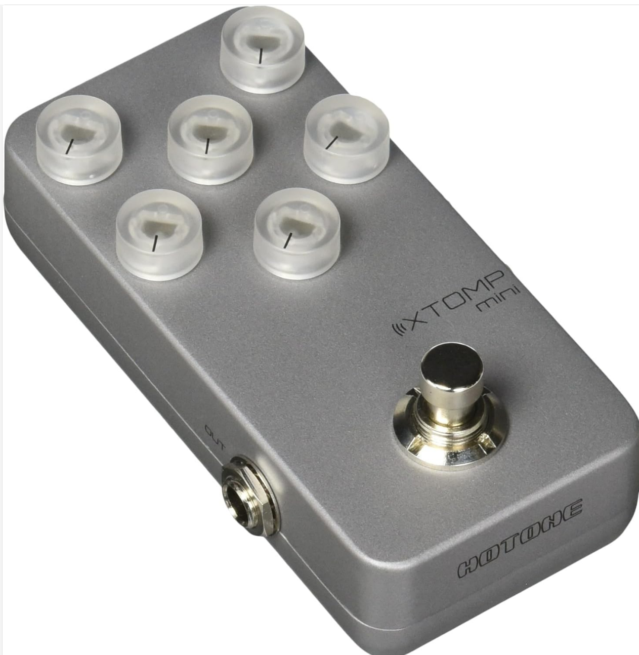
Image: Front view of the Hotone XTOMP mini, showing the input and output jacks on the sides.
