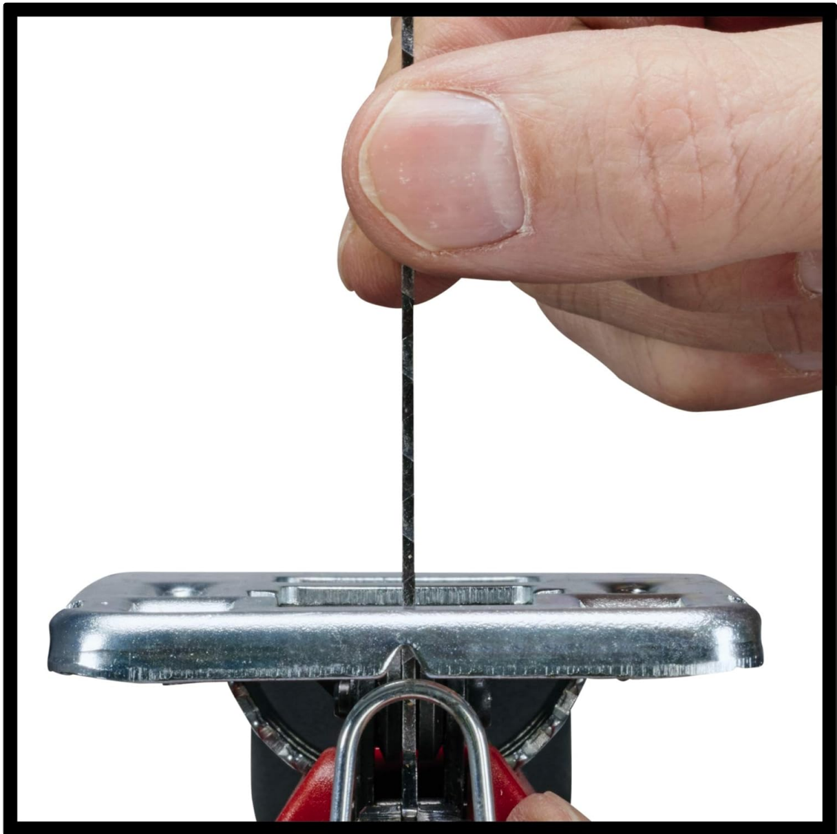
Image: A hand demonstrating the correct method for inserting a saw blade into the jigsaw's blade holder.
