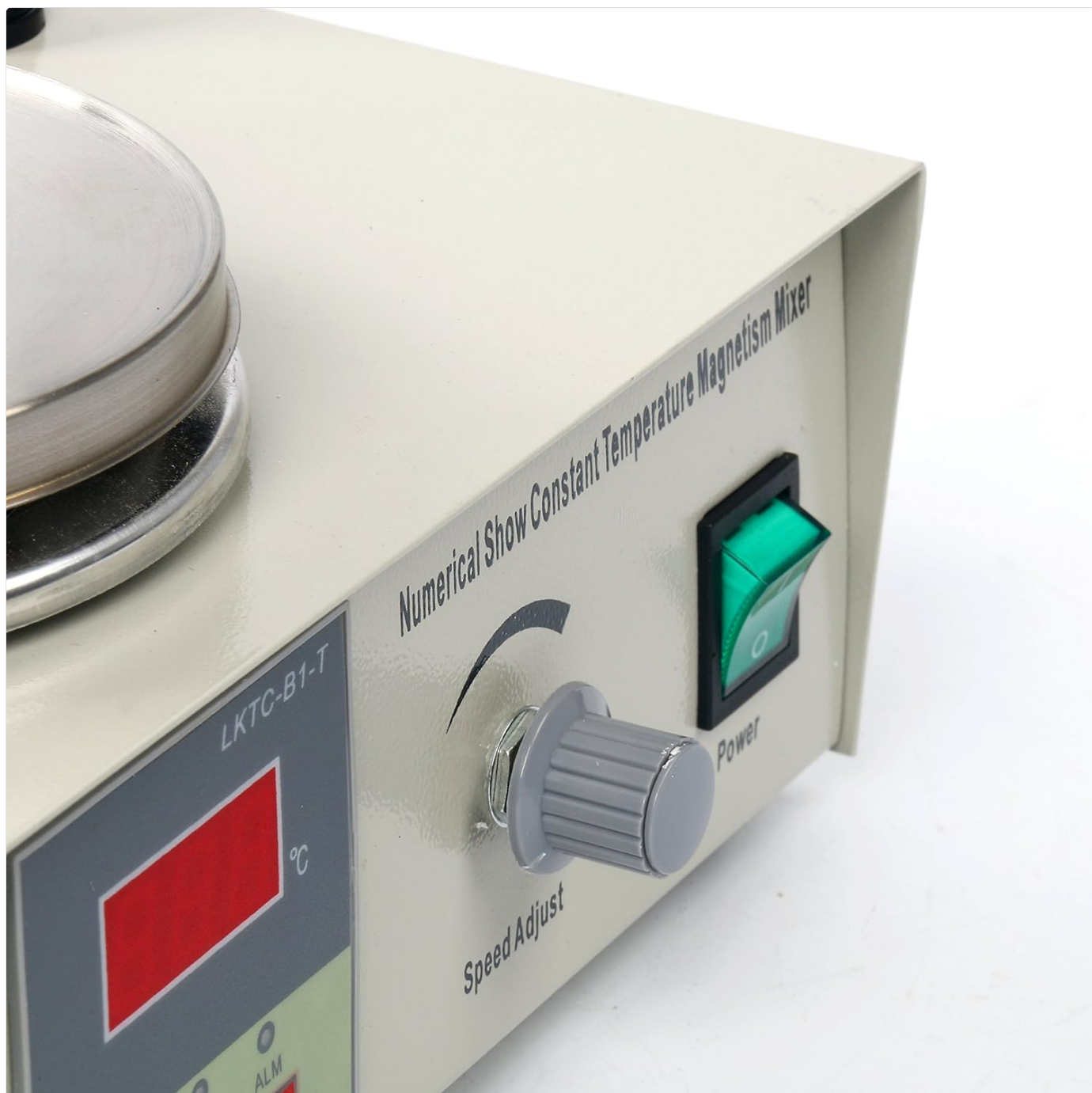
Figure 4.2: Detailed view of the "Speed Adjust" knob and the main power switch.
