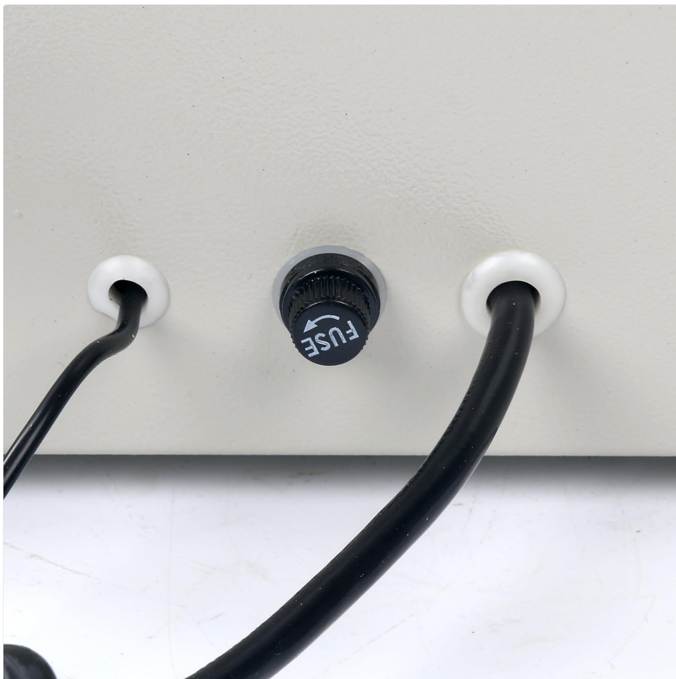
Figure 5.1: Location of the fuse holder on the rear panel of the unit.
