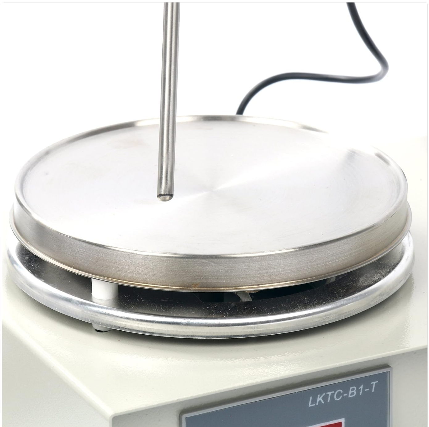
Figure 4.3: Close-up view of the stainless steel heating plate where the container is placed.
