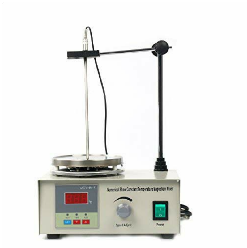
Figure 3.1: The magnetic stirrer hotplate fully assembled with the support stand and temperature probe in position.
