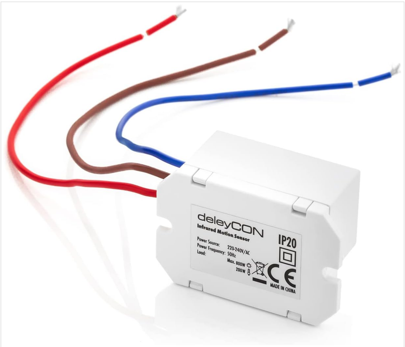
Figure 5.1: Wiring connections for the motion detector. Connect the live (brown), neutral (blue), and switched live (red) wires as indicated.
