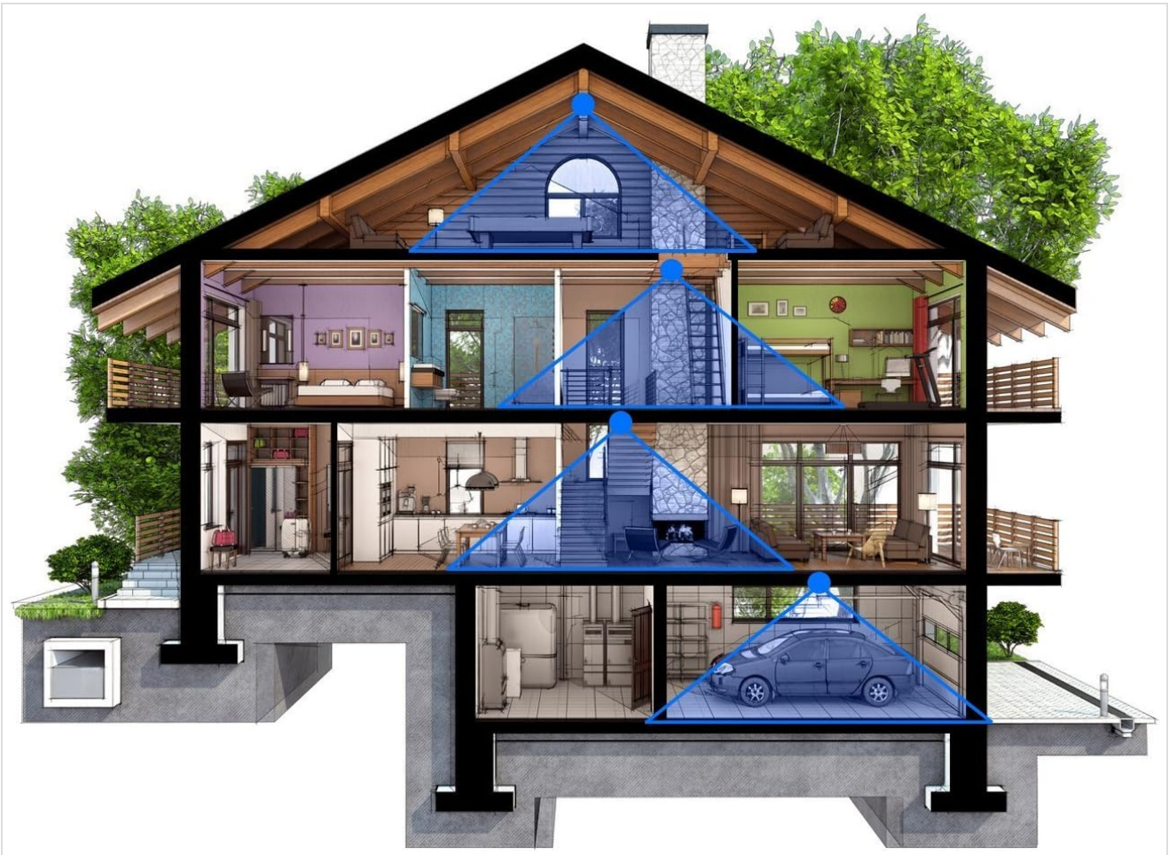
Figure 6.1: Example applications of the motion detector in various rooms within a house, illustrating its versatility for automatic lighting.
