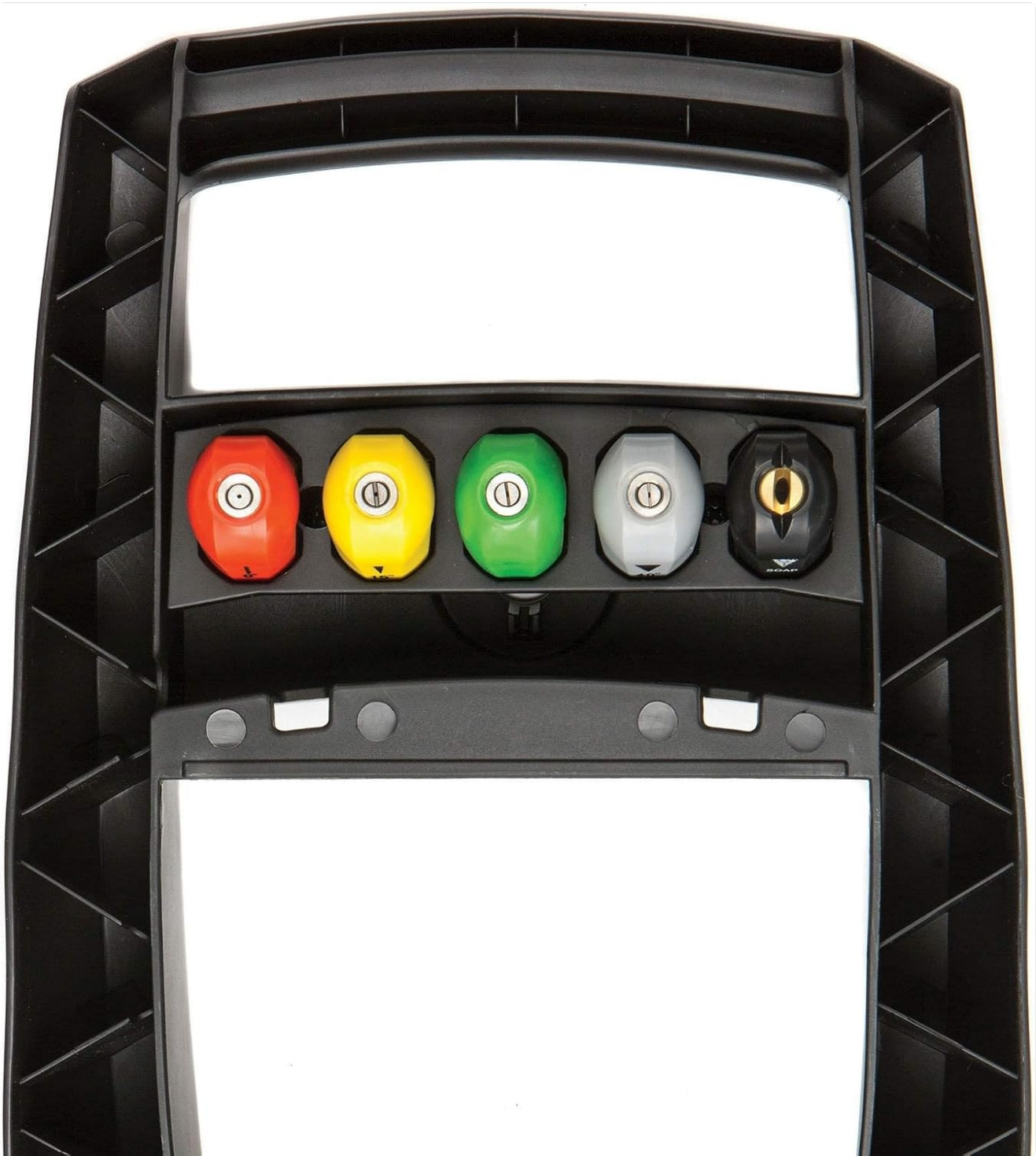
Figure 8: The five quick-connect nozzles (0°, 15°, 25°, 40°, and soap) for various cleaning tasks.
