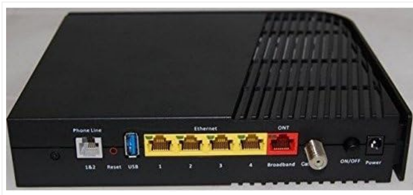
Figure 2: Rear view of the ARRIS NVG468MQ Wireless Gateway, displaying various ports including Ethernet, ONT, Phone Line, USB, and Power.
