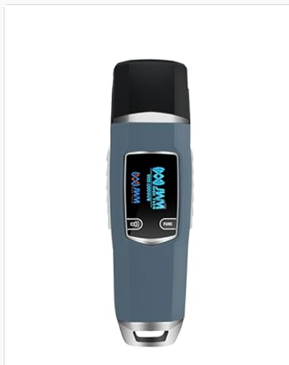
Image 2.2: The patrol reader's OLED screen and flashlight function.
