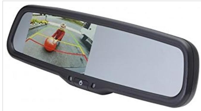
This image demonstrates the mirror monitor in operation, showing the integrated display with a camera view and overlaid parking guidelines, which assist in precise vehicle maneuvering.
