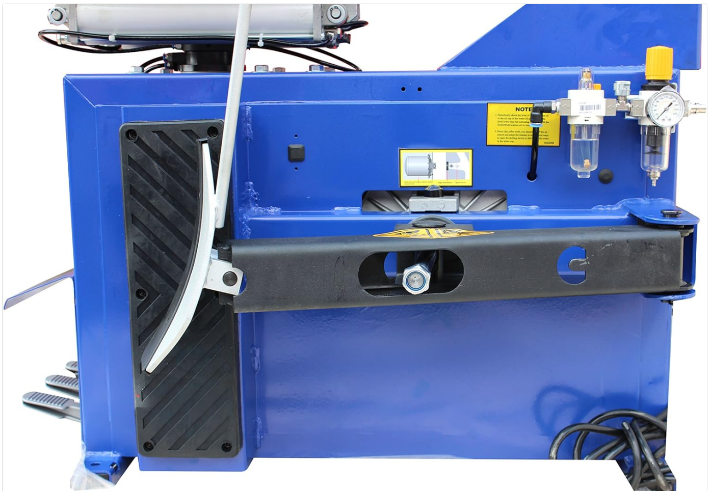
Figure 4: Side view of the tire changer illustrating air connections and pressure gauge.
