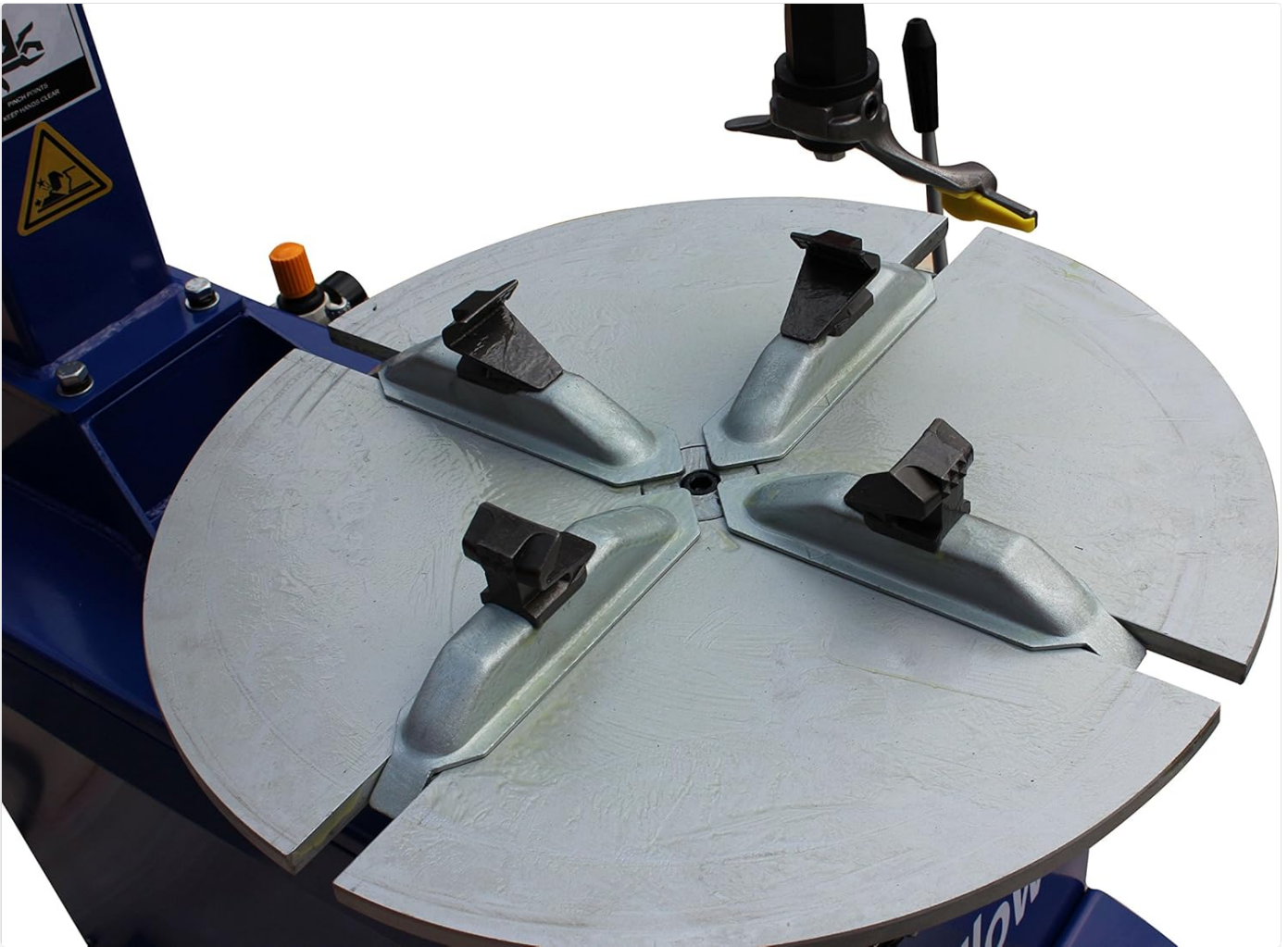
Figure 5: Close-up view of the rim clamping mechanism on the tire changer.
