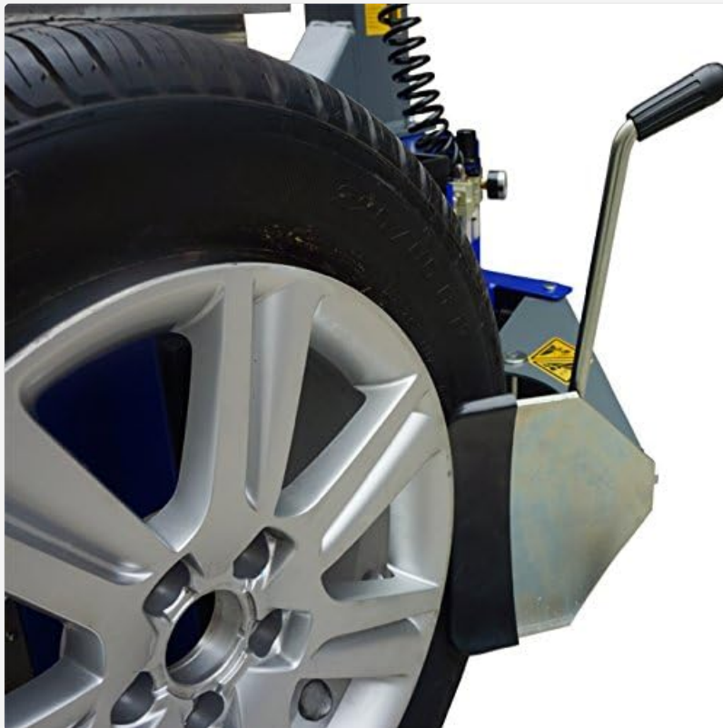
Figure 6: Close-up view of the bead breaker on the tire changer.
