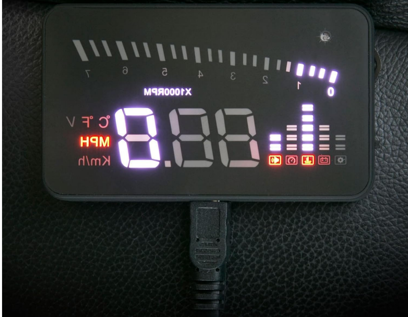
Figure 5: The HUD2 unit displaying indicators for programmable alerts.
