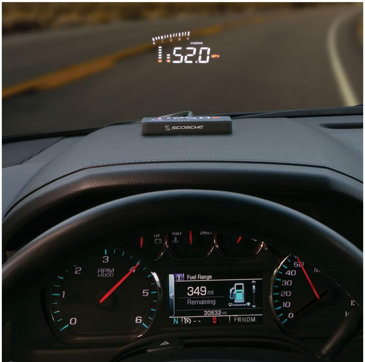
Figure 2: The HUD2 unit positioned on a vehicle dashboard, projecting information onto the windshield.
