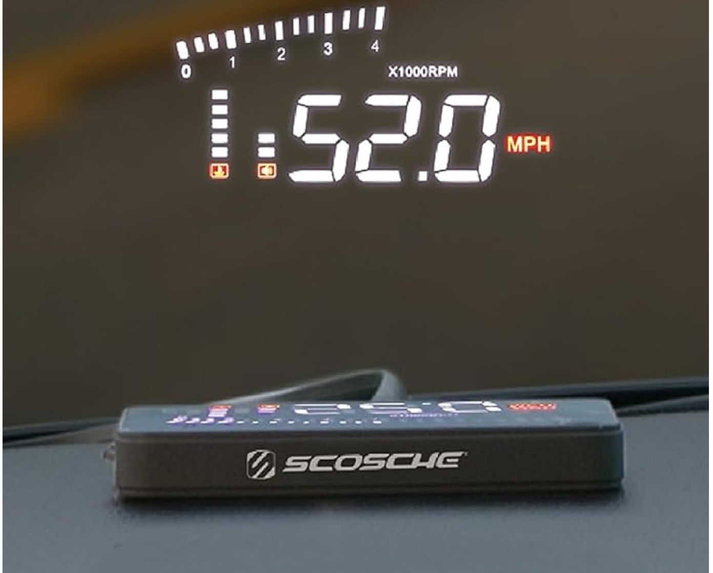
Figure 4: The HUD2 display aids in safer driving by projecting information directly onto the windshield.
