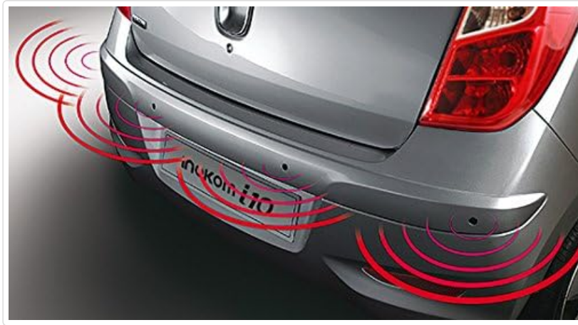
Figure 4.1: Illustration of the parking sensor system detecting obstacles behind a vehicle using ultrasonic waves.
