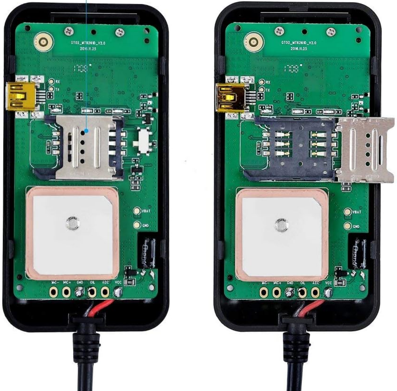
Image: A close-up view demonstrating the proper insertion of a standard SIM card into the designated slot within the Mbuynow GPS tracker's open casing.
