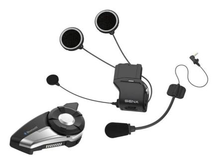
Image: All components of the Sena 20S-EVO-01D system, including the main module, speakers, and various microphone options.
