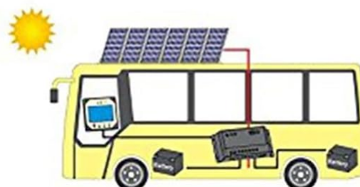
Figure 4: Example application diagram demonstrating the solar charge controller integrated into a bus system with solar panels and dual batteries.
