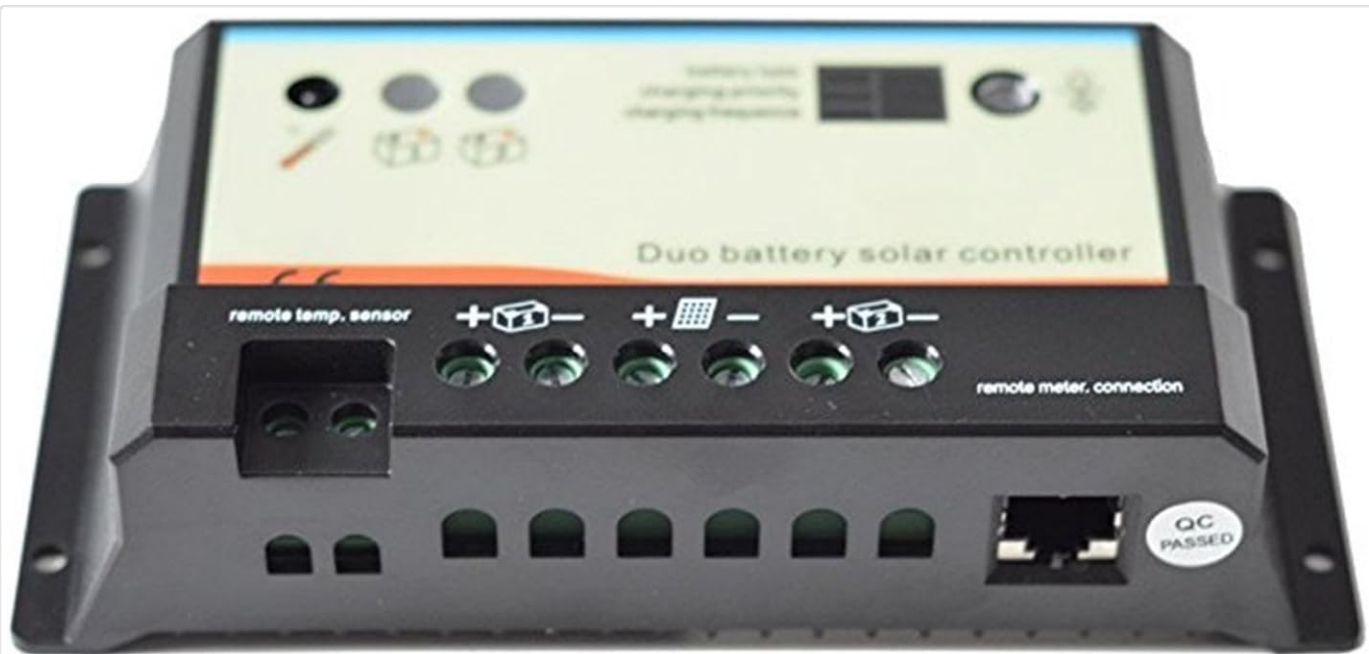
Figure 3: Side view of the controller, highlighting the connection terminals for batteries, solar panel, remote temperature sensor, and remote meter.
