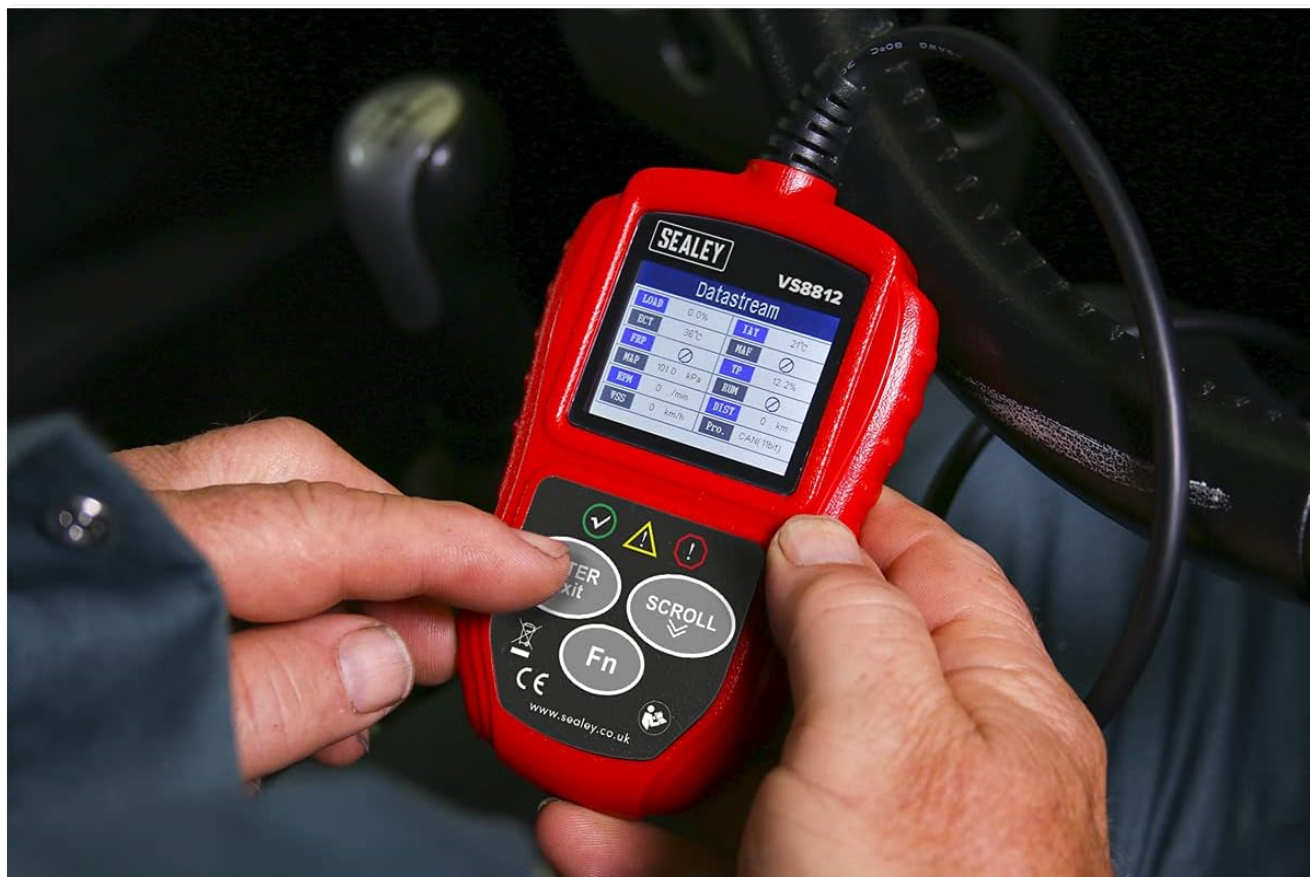
Figure 5.2: The Sealey VS8812 being used to display live data streams, showing various engine parameters such as LOAD, ECT, RPM, and vehicle speed.
