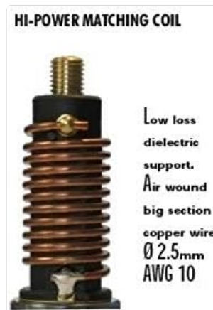
Figure 2.1: High-Power Matching Coil. This image shows the internal structure of the antenna's matching coil, featuring low-loss dielectric support, air-wound big section copper wire with a diameter of 2.5mm (AWG 10).
